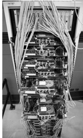
Figure 8.14. A Google server hosting multiple PCs. Clusters of server machines coordinate for searching to answer the user queries.
