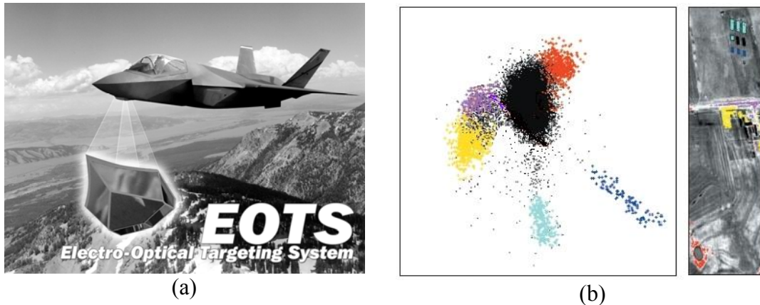
Figure 8.3 Hyperspectral dimensionality reduction for affordable spectral systems. (a) Electro-optical targeting system (b) Left. Hyperspectral Fisher discriminant subspace scatterplots showing color-coded target class clusters; Right. Hyperspectral image overlaid with color-coded target classes
